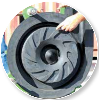
Schurco Hydraulic and Maintenance Training Seminar (Schurco 6x4 S Series natural rubber pump).
